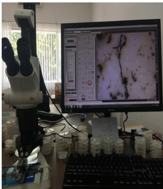
Fig. 4. S6D stereomicroscope integrated with a MC170 camera.
