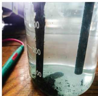
Fig. 4. Electrolyte product falling off the electrode.
