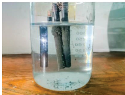
Fig. 11. Wastewater and electrode after treatment process.
