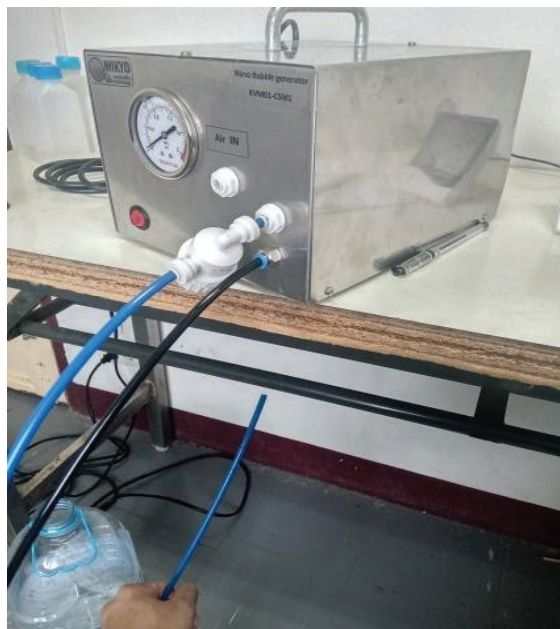
Fig. 1. Schematic diagram and image of the nano-bubble generator. The blue pipe is an inlet pipe in which water from the water tank and air from outside are absorbed. The black pipe is an outlet pipe, in which water carrying nano-bubble particles are released.
