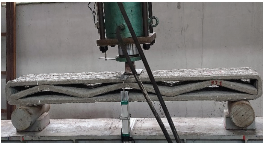
Fig. 15. Flexural test of triangle lattice model.
