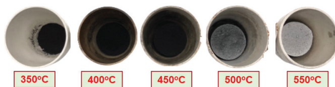
Fig. 2. Images of the biochar products obtained at different pyrolysis temperatures.
