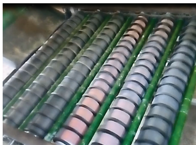
Fig. 2. Roller system of the carrot collecting machine.
