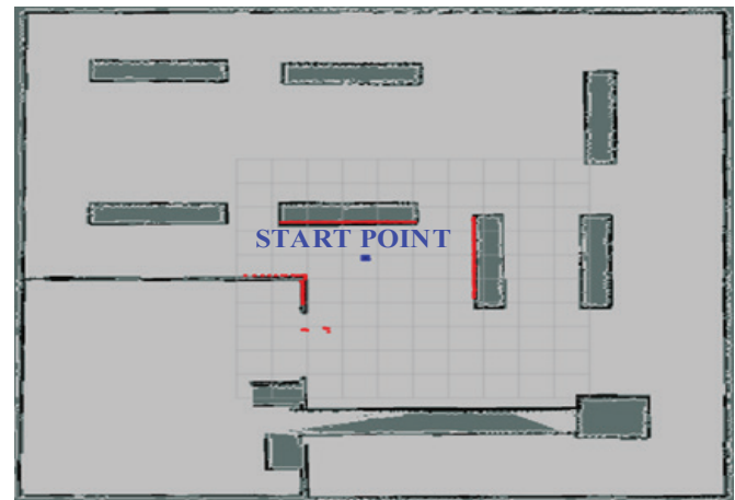
Fig. 8. Map obtained from the SLAM process.
