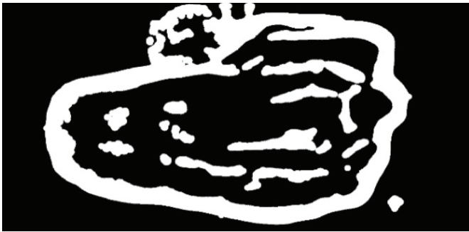
Fig. 5. Opening image. The circular structuring element has a diameter of nine pixels. The input image is Fig. 4B.
