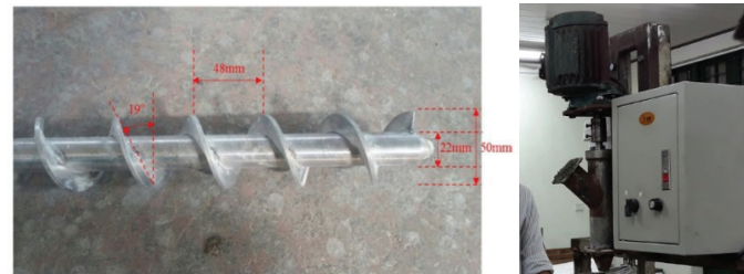
(A) Screw detail (used with permission from [14])
