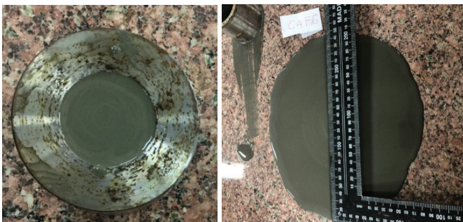
Fig. 3. Flow-slump of the tested binder.
