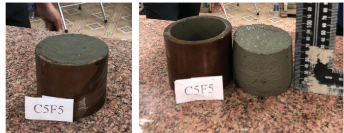
Fig. 5. The slump of the sample in the buildability test.
