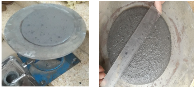
Fig. 1. Flow test apparatus and measurement of the flow diameter [15].
