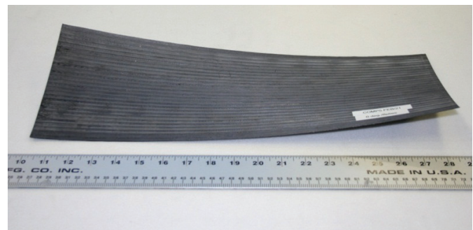
Fig. 14. Distorted flat plate, made from unidirectional layers [12].
