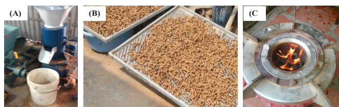
Fig. 3. (A) A pelletizing machine in an agricultural machinery company in Hanoi, (B) RS pellets produced, and (C) GCS-pellet cooking system demonstrated in Hanoi [52].
