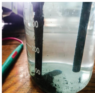
Fig. 4. Electrolyte product falling off the electrode.
