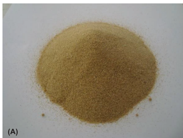
Fig. 2. Image of the poorly graded sand used in testing and its grain size distribution curve.
