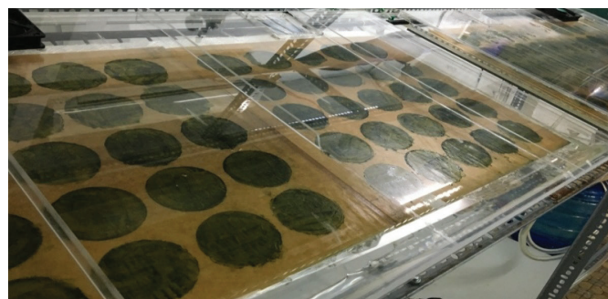
Fig. 3. Algae were immobilized into circular plots in angled TL-PSBRs.
