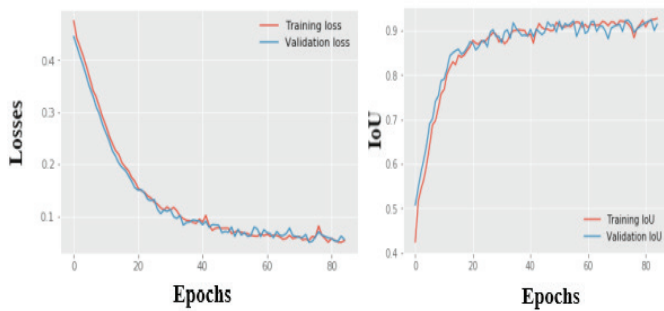
Fig. 6. Training and validation losses / IoUs of WBC segmentation model.
