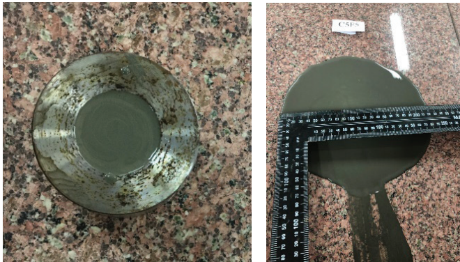
Fig. 3. Flowability of the tested binder.
