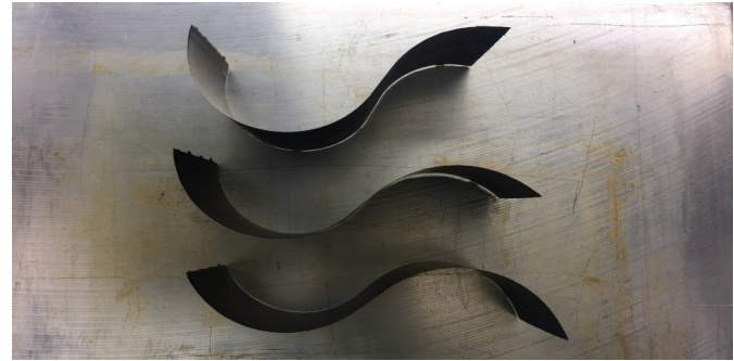
Fig. 4. Composite “S” shape made by 4DPC [10].
