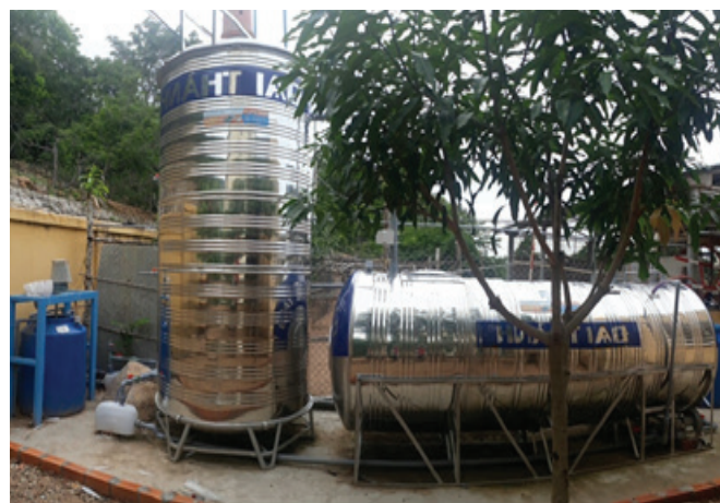
Fig. 1. The pilot scale AnMBR-CSTR model.
