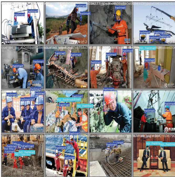
Fig. 12. Helmets detected by the proposed system on an outdoor construction site.
