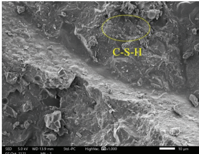
Fig. 12. Scanning electron microscopy micrographs of 28-day-old concrete.
