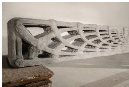
(B) Stress lattice struts [22, 27].
