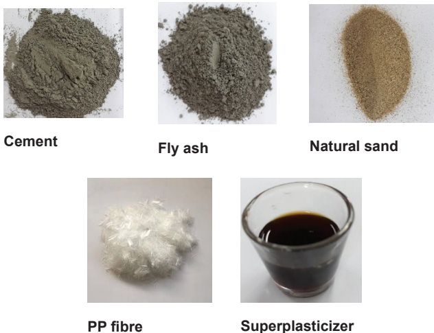
Fig. 3. Materials used for mixing concrete.
