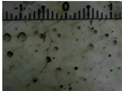
Fig. 5. A visual micro cracking network developing on the surface of the specimens containing 73% GGBS.
